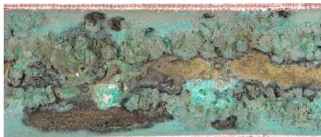
**Figure 1.** Longitudinal section of a water pipe after more than 10 years of use of copper/silver ionization. (Picture from Boffardi BP, Hannigan JM. A limited evaluation of pitting corrosion of copper piping in a hospital domestic hot water system using copper-silver ionization for *Legionella* control. AWT, Mohegan, 2013.)
